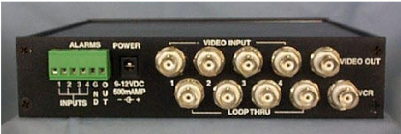
LEDs on the front of the QS-402HR. The green one to the far left will be illuminated continuously when power is applied. Next connect the four BNC video inputs to the unit from the cameras or video sources. As seen above they are labelled 1-4 corresponding to the four front panel buttons. The two BNCs to the left are the video outputs and should be connected to the video monitor. If connected directly to the video monitor and no other looping devices then this monitor should
