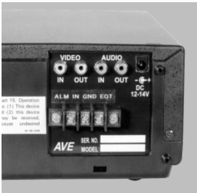
The RT-195 requires the use of composite video. To see the on-screen programming menu, you must have a video camera in and a monitor connected.
