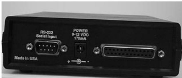
**Figure 1a.** P2RS Parallel to Serial Converter
