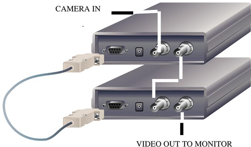
**Figure 16:** Down Load Set Up Between VSI-Pro and VSI-Pro
