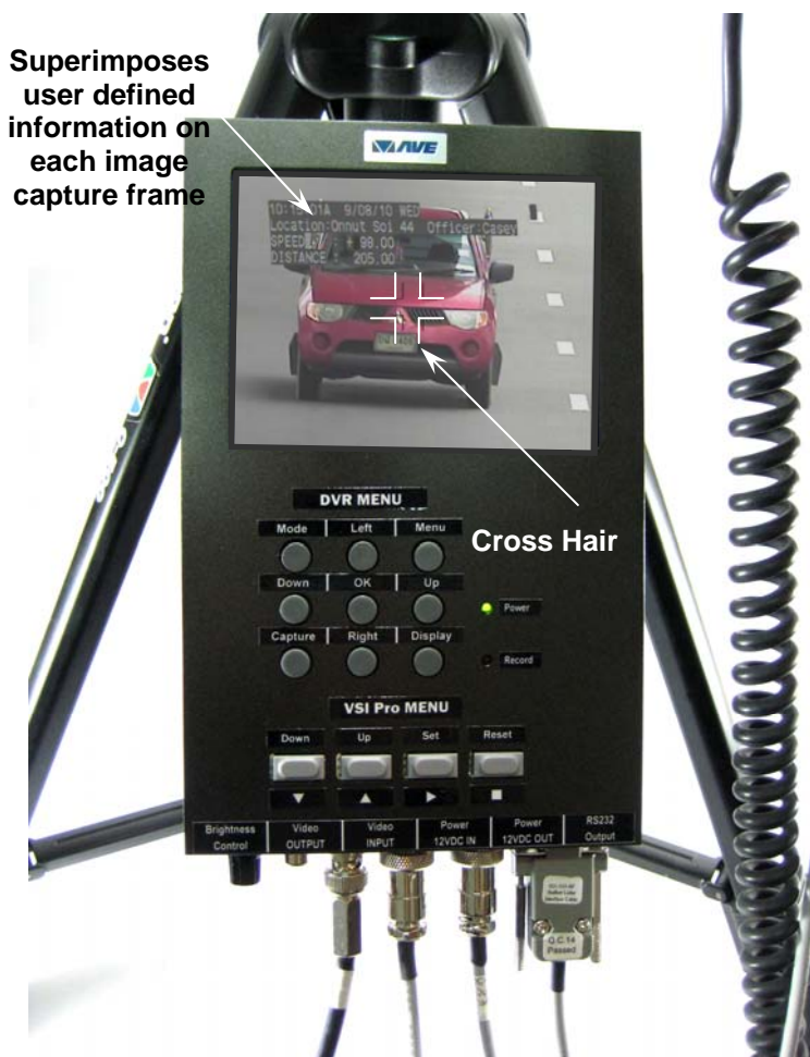
◀ Figure 2.0 Portable Speed DVR System
