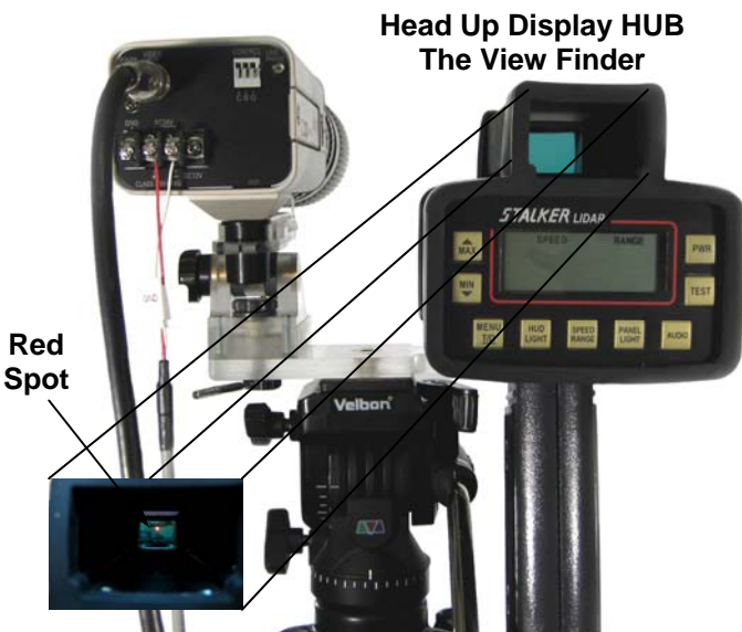
◀ Figure 1.0 Stalker Lidar Speed Gun
