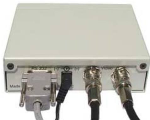
Serial Input Power Video Input Video Output Figure 3: VSI-Pro Radar Cable Connections
