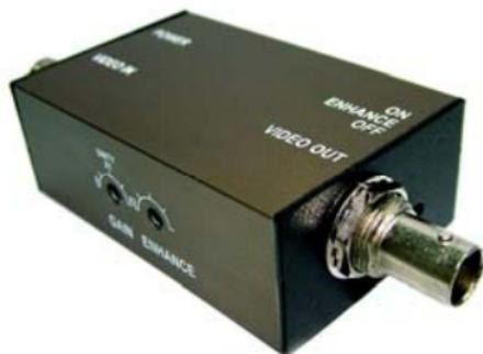
The VECA is an inline device to pre-compensate for video degradation due to long cables designed to be mounted at the head end or the camera side. There are two controls on the VECA, one for Enhancing and the other for Gain.
