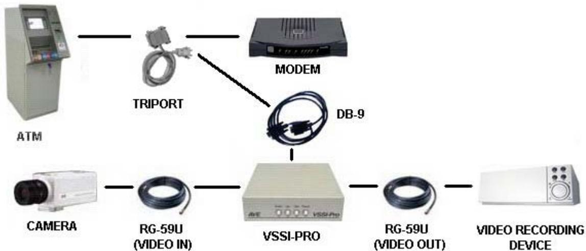
Figure 1: Typical VSSI-Pro Connections
