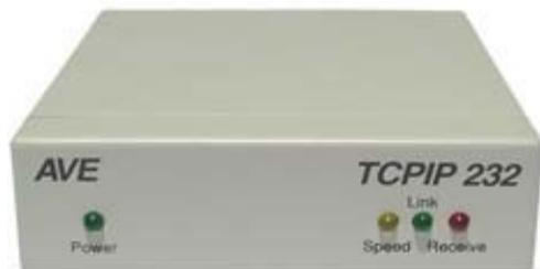
Figure 15: Front of TCPIP 232 Adapter
