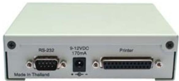
Figure 2B: P2RS Parallel-to-Serial Converter Rear Panel
