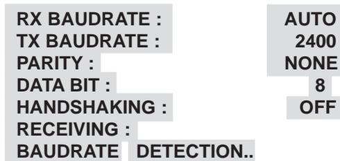
Figure 71: RECEIVE [ RX ] TEST Display
