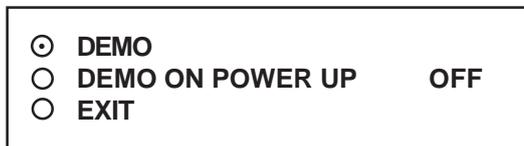
Selecting “DEMO” will give you two options of 19 or 37 characters per line. After selection the demo will start after a few seconds. To exit this demo, press and release “Reset”. If data is sent to the VSI-Pro during this demo mode with “DEMO ON POWER UP” set to OFF then the demo mode will be disabled and you must go back into the programming mode and select again as described above.
