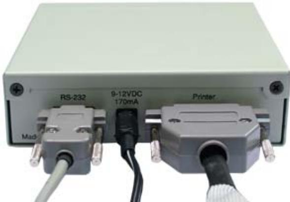
Serial Input                  Power                  Printer Cable
